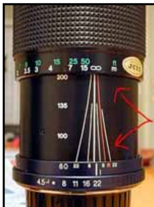
Older lenses including zoom lenses, have DOF markings as indicated by the red markers
