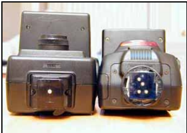
The Vivitar 283 hotshoe compared to the TTL Nikon SB28 hotshoe - one hot pin versus four hot pins on the Nikon
