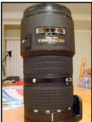
Current autofocus zoom lenses do not have DOF markings anymore
