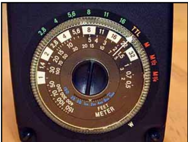
The Calculator and Mode Dial on a Metz 45 CL-4 - the green aperture settings are for the Auto flash mode
